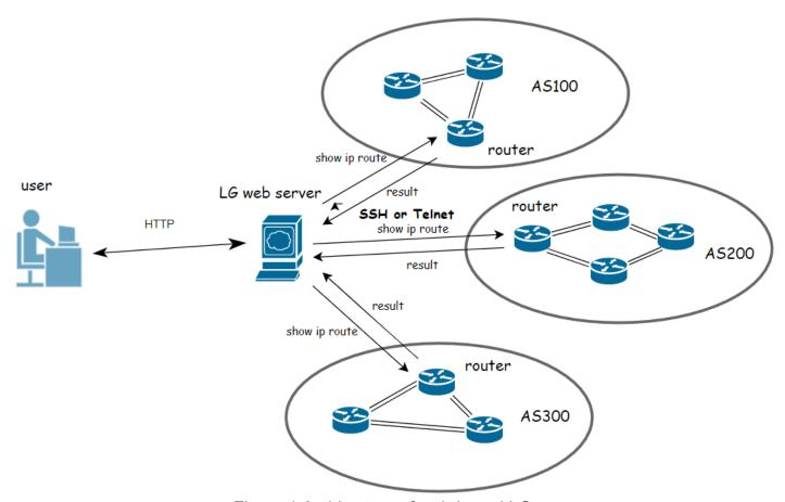
Figure 1 Architecture of web-based LG
