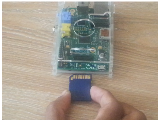
Figure 8: installing SD card
