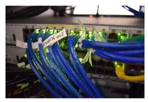
Our four new HP ProCurve switches (two of which were procured from the grant) are OpenFlow compatible and give us the option of reshaping the behaviour of the wold-side network of the simulator.
