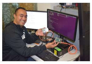
Fuli works on non-connection-breaking PEP software that we will hopefully be able to deploy on the simulator next year. He uses two Raspberry Pis and a PC to emulate a small network.
