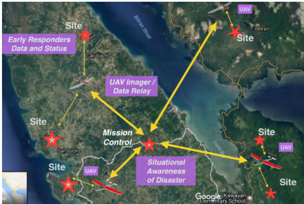
Figure 6. The use of UAVs as data ferries in an information system to provide situational awareness
